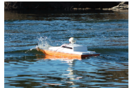
Fig1. Remote controlled boat completes a dam survey.
